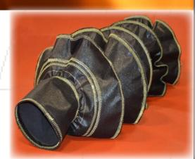
THERMOPAK® ROBOT COVERS are made with ARMATEX® SBN 13-602 Robotex, a unique, lightweight silicone coated fabric designed to maintain flexibility, and retain chemical and thermal stability in high temperature environments. Constructed with an aromatic polyamide base fabric that has exceptionally high strength and crystallinity, this fabric can be used in applications that require high tensile strenth and high flexural failure resistance.
