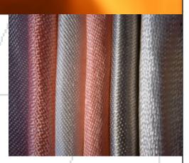
Fire barriers constructed from HYTEX® 2500 are lighter weight than metallic materials, and have successfully passed FAA 2000°F • 1095°C 15 minute flame penetration tests. Low thermal conductivity and high electrical resistivity makes these textiles highly efficient as high-temperature barriers and electrical insulation.
