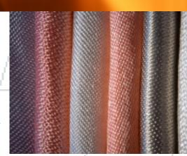
Fire barriers constructed from HYTEX® 2200 are lighter weight than metallic materials, and have successfully passed FAA 2000°F • 1095°C 15 minute flame penetration tests. Low thermal conductivity and high electrical resistivity makes these textiles highly efficient as high-temperature barriers and electrical insulation.
