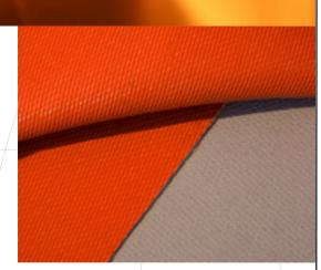
Other applications include use in weld splatter protection of equipment and personnel, as well as heat shields, splash curtains, and thermal insulation barriers.
