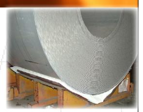
THERMOPAK® TRAY PADS can also reduce in-house scrap on CSA (contact surface abrasion) and bruising by 60% or more by eliminating steel to aluminum contact while transporting, annealing and handling both hot and cold aluminum coils, slab, sheet, billett, and extrusions.
